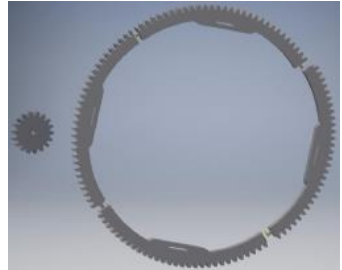
Figure F: 3D gears drawn in AutoDesk Inventor
