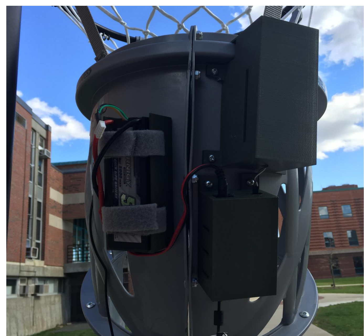
Figure H: 3D casings mounted to the back of the funnel.
