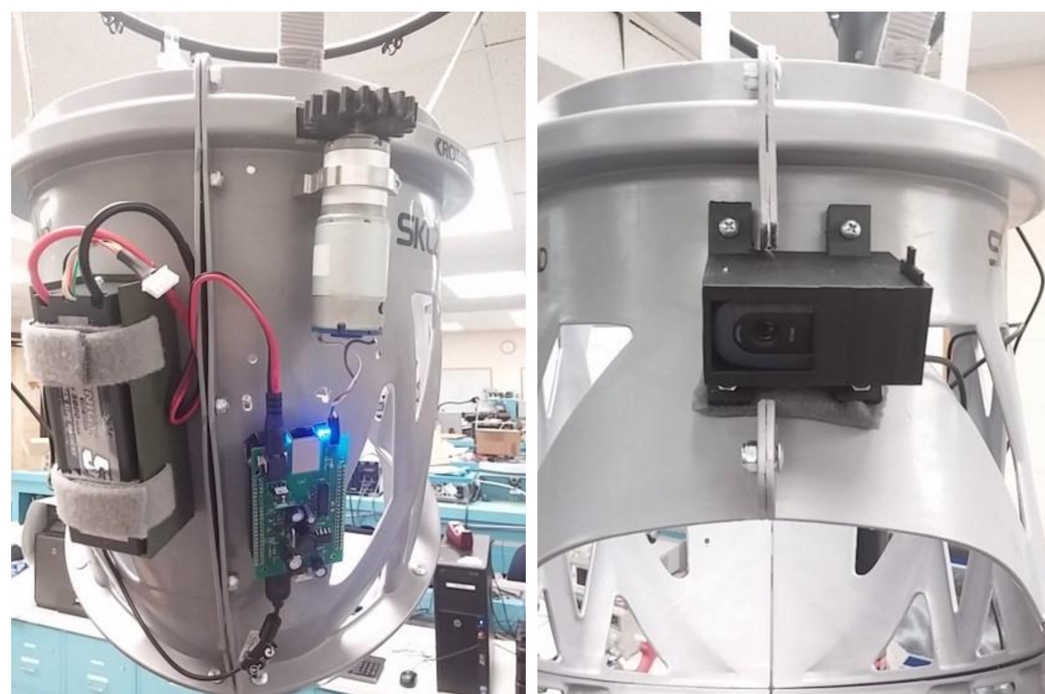
Figure B: Battery powering the BeagleBone and motor (left) and webcam mounted (right).
